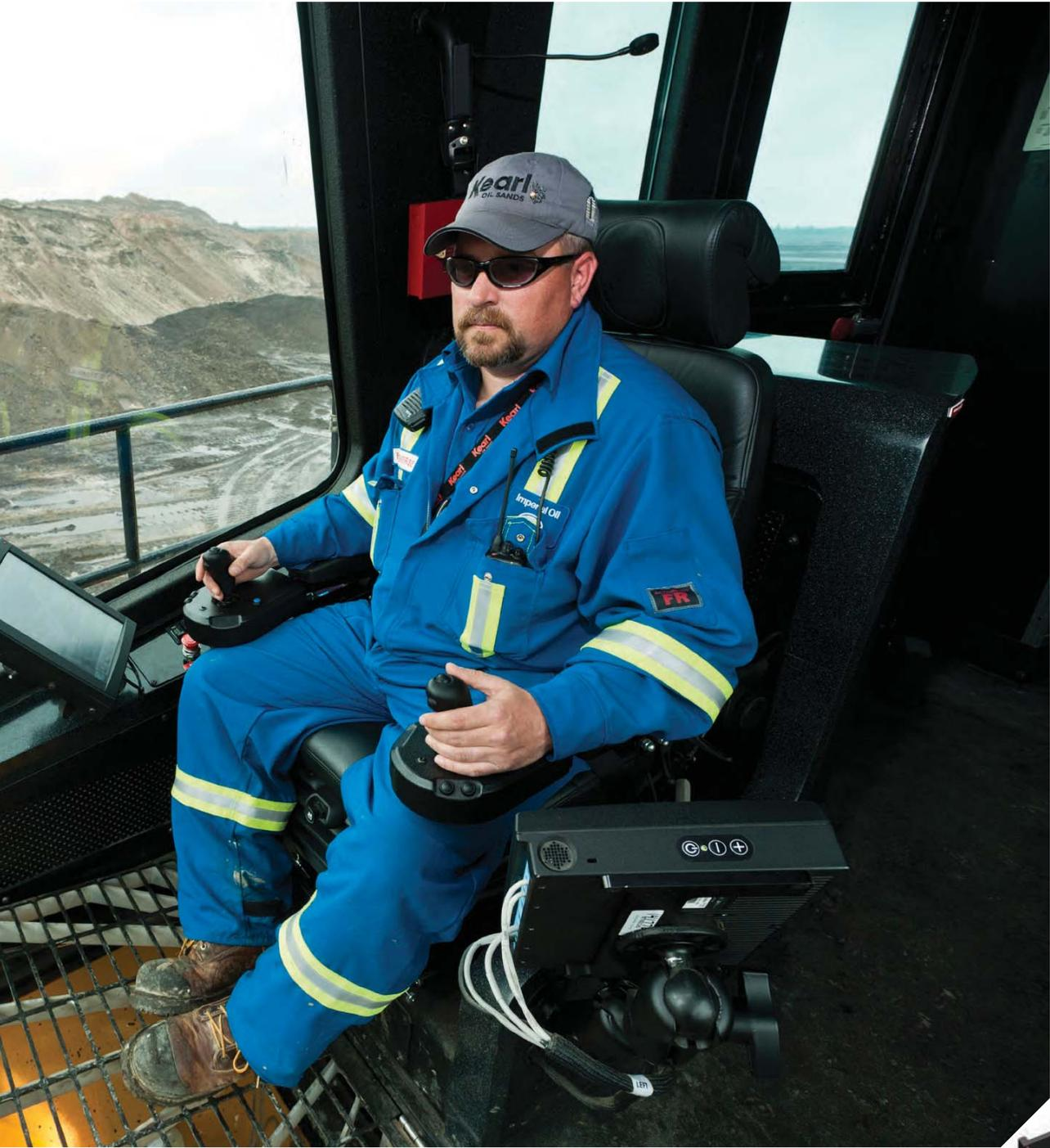
**MAIN IMAGE:** With 12-hour shifts the norm in mining shovels and draglines, a brand-new cab design that met the functional needs of the operator, as well as his 'habitational' needs, was a key requirement
