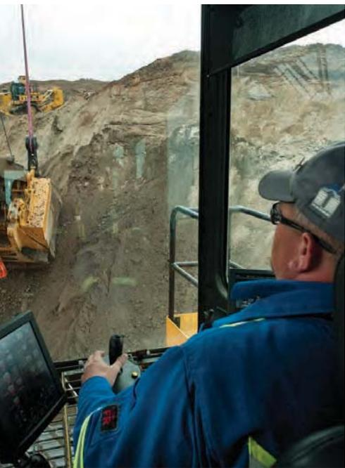
Designing the operator's station was a major undertaking in its own right. Special emphasis was given to having a fully adjustable seating and armrest system to accommodate the full range of operators as they ran controls while experiencing a considerable amount of motion.
